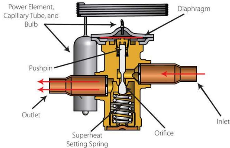
Thermal expansion valves are robust, simple, and inexpensive. The electronic expansion valves are more expensive but offer greater level of control in the refrigeration circuit. This affords the system designers the ability to optimize the performance for greater performance and reliability.
