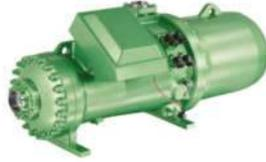
**Screw compressors** also use positive displacement to compress the refrigerant. The compressor uses two meshing screw-rotors. These rotate in opposite directions to increase the refrigerant gas pressure. Screw compressors require oil for lubrication. Screw compressors can be disassembled for maintenance and repair.
