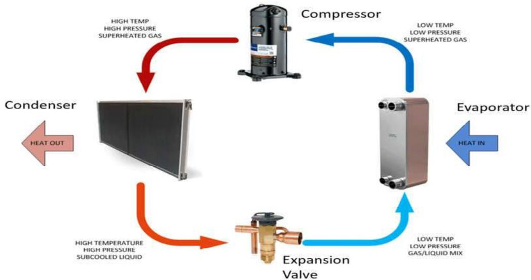
[The Refrigeration Cycle – the process of heating and cooling the refrigerant and changing it from a gas to a liquid and back again is the refrigeration cycle.](#)
