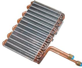
**Coil heat exchangers** are most often air-to-water or air-to-refrigerant units. These consist of tubes with fins stacked together to form flat pieces. A common example of a coil heat exchanger is a radiator in a car. Forced air through the coil's fins conduct heat from the fluid in the tubes, through the fins and into the air. These are often condensers in air-cooled chillers.
