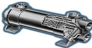
**Shell and Tube Heat Exchangers** use an outer shell vessel with internal tubes to isolate the two fluids. Large passageways between the tubes inside the shell avoid clogging but this reduces the efficiency of heat transfer. Shell and tube heat exchangers are commonly used in applications where one of the fluids contains high levels of contamination. Variations of these heat exchangers are used as condensers in water-cooled chillers.
