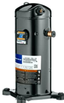
**Scroll compressors** use positive displacement to compress the refrigerant from a low pressure gas to a high pressure gas. The compressor motor is cooled by refrigerant passing over it. Oil is a critical component of a scroll compressor for lubrication. Scroll compressors are hermetically sealed and often replaced rather than repaired.
