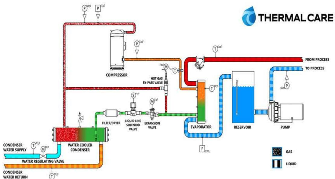
**Compressor** is a vessel used to increase the pressure and temperature of refrigerant gas and circulate it through the process cooling system.
