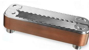
**Brazed plate heat exchangers** are a variation of the plate and frame design. The plate pack is permanently brazed together. This eliminates the need for the frame, gaskets, and end plates. This design improves the efficiency over a standard plate and frame. These are also much more compact but are not easily cleaned. Brazed plate units are often used as evaporators in chillers.
