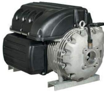
**Centrifugal Compressors** are dynamic and raise the refrigerant pressure by rotating an impeller. This creates centrifugal force which compresses the gas. Certain centrifugal compressor designs, like those on the Thermal Care TC and TCF series, use magnetic bearings and do not require any oil for lubrication. Centrifugal compressors can be disassembled for maintenance and repair.
