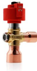
**Hot gas bypass valve** is used for capacity control of a chiller. It provides an artificial load on the evaporator by introducing high pressure, high temperature gas to the evaporator. This prevents the compressor from short cycling the system when the demand for cooling is low. Additionally, the hot gas keeps the evaporator from freezing and prevents low refrigerant pressure alarms.
